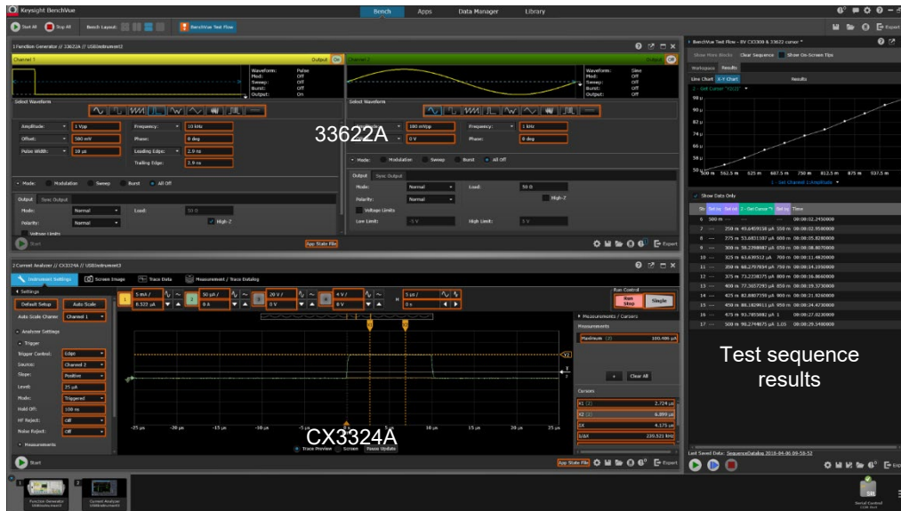
Figure 23. BenchVue test sequence using a Keysight 33622A waveform generator and a CX3324A to make a simple pulse measurement
