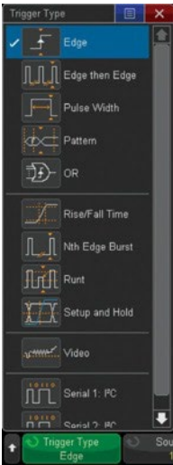
Figure 41. Wide array of advanced parametric trigger modes.
